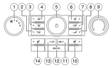
1. **Fan speed adjustment:** Turn to select fan speed.
